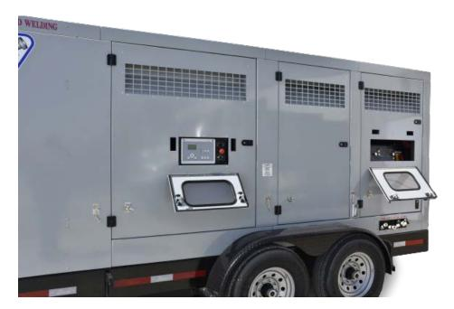
The stud welder compartment door and the generator operations panel door are equipped with small glass fronted access doors so that the main doors don't have to be opened during operation of the generator to facilitate changes for the stud welder or generator when necessary.
