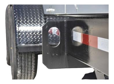
The generator system has four (4) lifting points for easy and safe handling when it is required to lift the unit by crane. Any two (2) diagonal hooks can support the weight of the entire unit safely.
