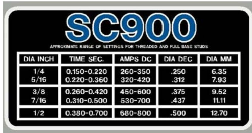
The image shows a settings chart for the SC900 machine. The chart is titled "SC900" in large blue letters, with "APPROXIMATE RANGE OF SETTINGS FOR THREADED AND FULL BASE STUDS" written below it. The chart is a table with five columns: DIA INCH, TIME SEC., AMPS DC, DIA DEC, and DIA MM. The rows represent different stud diameters: 1/4, 5/16, 3/8, 7/16, and 1/2 inch.
