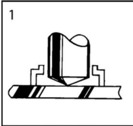
1 The weld gun is positioned over the base material and the main gun spring is partially compressed. Hold gun perpendicular to work surface and hold ferrule firmly against the surface.
