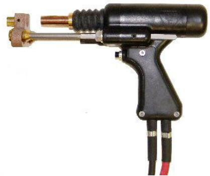
The SC900 is a fully integrated stud welding system for ferrule-shielded and gas-shielded drawn arc stud welding. The SC900 contains digital controls for weld time, weld current, and gas purge time. The system was designed to be a perfect fit for shop use, welding up through 1/2" studs. This is all contained in a compact, portable package.
