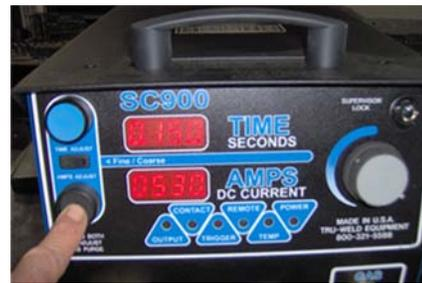
When setting time or current, depress and hold down appropriate button, and turn Adjustment Dial clockwise or counter-clockwise to the correct setting on the digital display.
