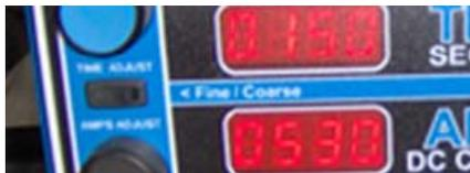
To adjust gas purge time, hold both the TIME and AMPS buttons and turn Adjustment Dial. The setting is saved when the buttons are released.
