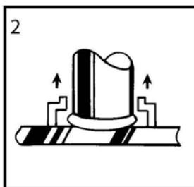
2 The trigger is pressed and the stud lifts off the base, drawing an arc. The arc melts the end of the weld stud and the base material below. The arc shield (ferrule) concentrates the heat below the weld stud and contains the molten metal within the weld zone. Do not move weld gun during weld.
