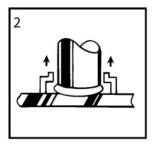
The trigger is pressed and the stud lifts off the base, drawing an arc. The arc melts the end of the weld stud and the base material below. The arc shield (ferrule) concentrates the heat below the weld stud and contains the molten metal within the weld zone. Do not move weld gun during weld.
