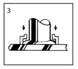
The main spring plunges the weld stud down into the molten pool of metal in the base material. The cycle is completed in less than a second and the resulting weld bond develops the full strength of the fastener in the weld zone. Allow metal to cool and withdraw gun from the stud, pulling the gun straight up off of the stud.
