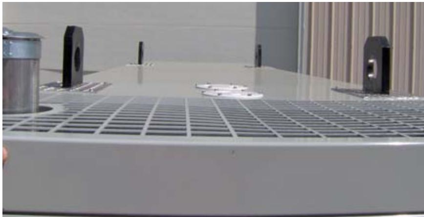
The generator system has four (4) lifting points for easy and safe handling when it is required to lift the unit by crane. Any two (2) diagonal hooks can support the weight of the entire unit safely.
