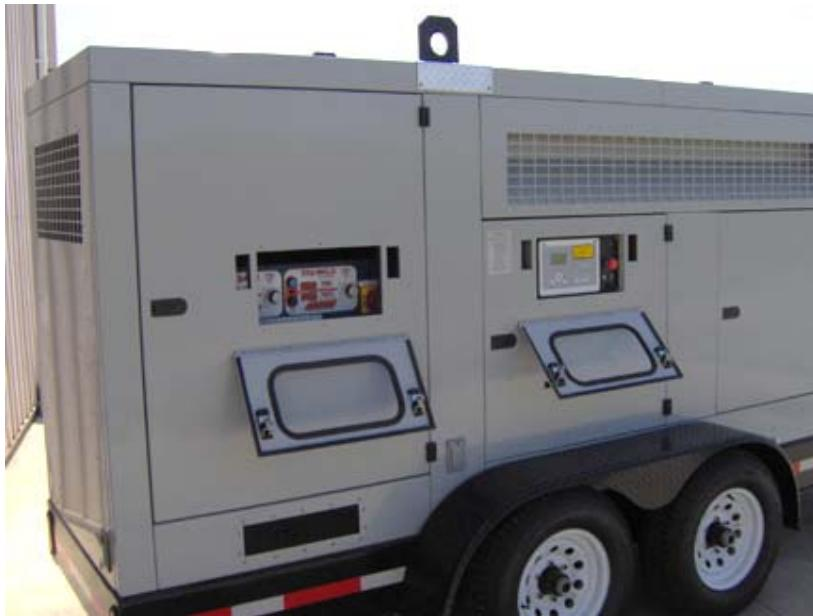
The stud welder compartment door and the generator operations panel door are equipped with small glass fronted access doors so that the main doors don't have to be opened during operation of the generator to facilitate changes for the stud welder or generator when necessary.
