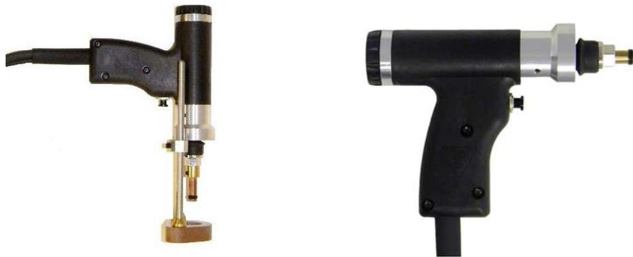
When removing the stud gun from the welded stud, always lift the stud gun vertically from the welded stud in order to maintain the proper tension of the collet. Spreading the collet when lifting the stud gun from the welded stud will shorten the life of the collet and will eventually create an undesirable weld.
