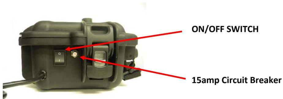
The controller ON/OFF switch is located on the rear of the unit in the upper right hand corner. Below this switch is the 15amp circuit breaker for the system.
