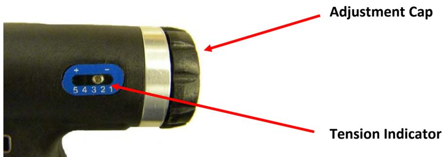
This spring pre-load adjustment is made by turning the adjustment cap on the back of the stud gun. On the bottom of the back cap of the stud gun is the indicator numbered 1 thru 5, which will show you the tension setting during the adjustment.
