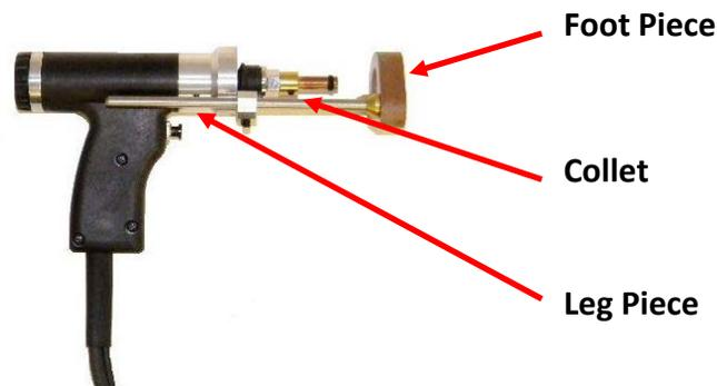
When the legs and foot piece are in place, insert the stud to be welded into the collet. Adjust the leg and foot piece by sliding it into position until approximately 1/8” of the stud protrudes from beyond the foot piece. Lock legs in place with the set screws.
