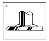
The weld gun is withdrawn from the weld stud leaving and the ferrule. The ferrule is broken away and discarded. Visually inspect weld.
