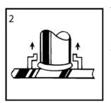
The trigger is pressed and the stud lifts off the base, drawing an arc. The arc melts the end of the weld stud and the base material below. The arc shield (ferrule) concentrates the heat below the weld stud and contains the molten metal within the weld zone. Do not move weld gun during weld.
