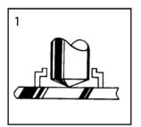
The weld gun is positioned over the base material and the main gun spring is partially compressed. Hold gun perpendicular to work surface and hold ferrule firmly against the surface.
