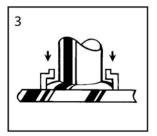
The main spring plunges the weld stud down into the molten pool of metal in the base material. The cycle is completed in less than a second and the resulting weld bond develops the full strength of the fastener in the weld zone. Allow metal to cool and withdraw gun from the stud, pulling the gun straight up off of the stud.
